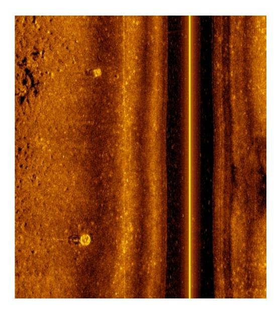
Figure 1. An example of a sidescan sonar image of derelict crab pots. (Square sport pot in upper image and round commercial pot with line in lower image). Source: Innerspace Exploration Team.
