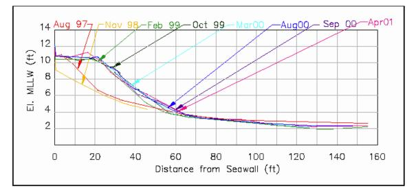
Figure 8. Profile 9, near west end (down-drift end) of Samish Island protective berm, looking west.
