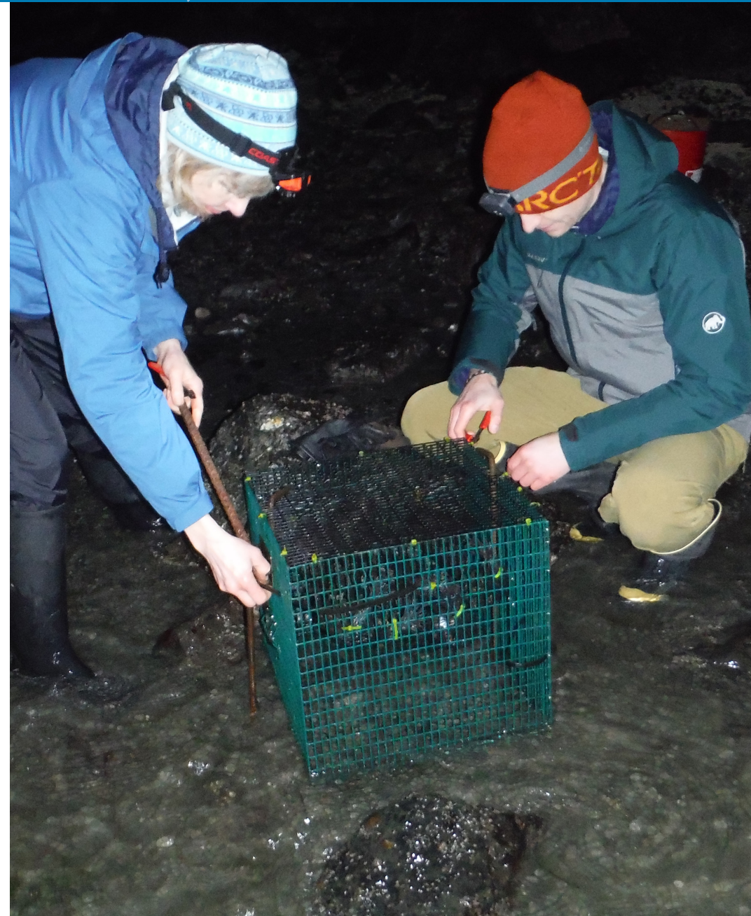
Caged mussels are safely anchored in the Sound and retrieved 3 months later for pollutant analysis.
