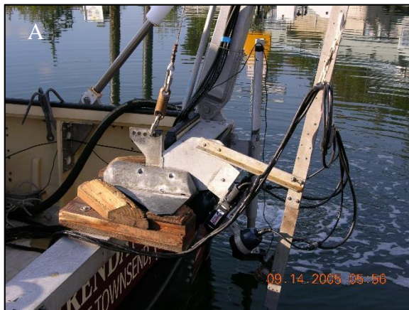
Figure 2: The R/V Brendan D II is equipped with a weighted towfish that contains an underwater video camera mounted in a downward looking orientation, dual lasers for scaling reference, and underwater lights for night work (A). The towfish is deployed directly beneath the DGPS antenna attached to the A-frame cargo boom, ensuring accurate geographic location of the camera (B).
